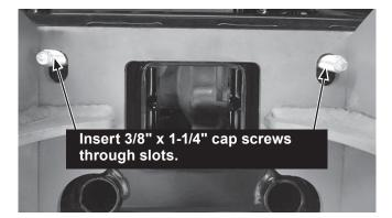
Secure cap screws with 3/8" washers and 3/8" locknuts. Hand tighten the fasteners.
