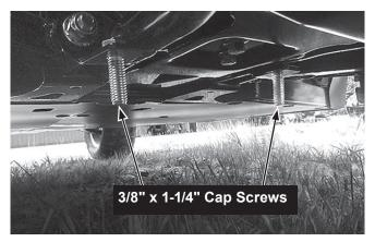
6. Install 3/8" washers on two 3/8" x 1-1/4" cap screws. Insert the cap screws with washers through the slots on the front of the vehicle.
