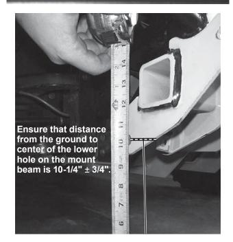
Measure the distance between the mount beam rear hole and the ground. If it exceeds 11-1/2", install the accessory Height Adapter Plate Kit (PN 77555) to ensure optimum plowing performance.
