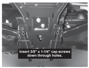
5. Place the skid plate assembly against the vehicle frame, allowing the fasteners installed in Step 3 and Step 4 to pass through the assembly. Secure all four cap screws with 3/8" locknuts; hand tighten.
