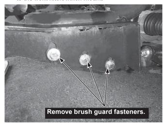
10. Loosen the two upper brush guard fasteners.
