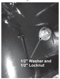
6. Tighten all fasteners according to the torque chart, starting at the front of the vehicle.
