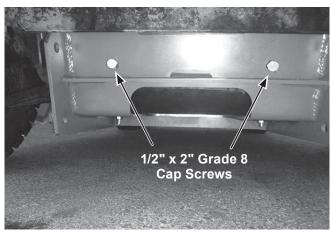
Secure the cap screws with 1/2" washers and 1/2" locknuts. Hand tighten the fasteners.
