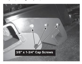
Secure the cap screws with 3/8" washers and 3/8" locknuts. Hand tighten the fasteners. Repeat on the passenger's side.
