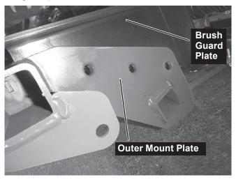
Secure the mount assembly to the skid plate assembly using four 1/2" x 1-1/4" cap screws and 1/2" locknuts. Hand tighten the fasteners.
