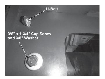
Secure the cap screws with 3/8" washers and 3/8" locknuts. Hand tighten the fasteners.
