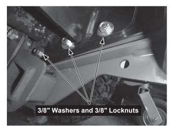
14. Tighten all fasteners according to the torque chart.
