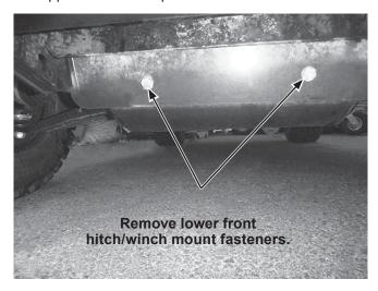
2. Ream the two lower holes of the front hitch/winch mount and the corresponding holes on the vehicle to 17/32".
