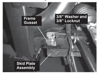
12. Ensure that the frame gusset is pushed against the frame rail. Use the hole in the bracket as a guide to drill a 3/8" hole through the frame rail.
