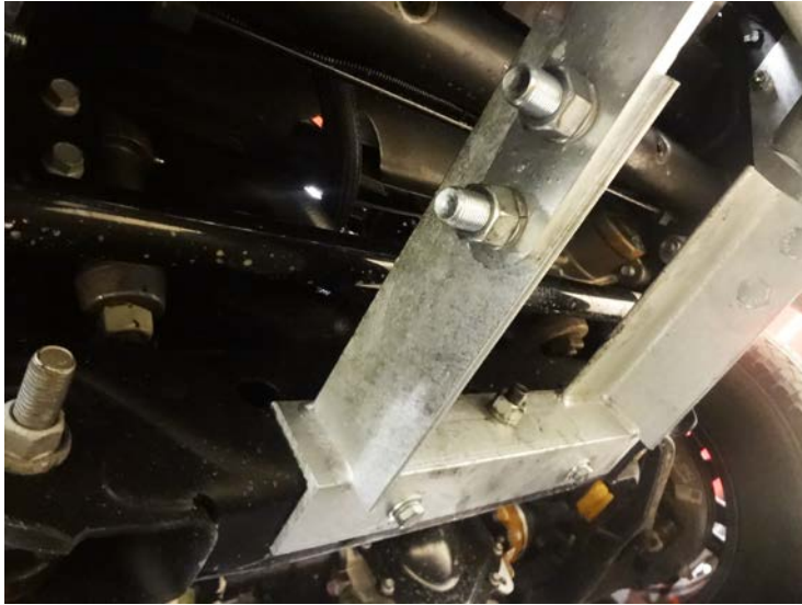
Thrust arms (2) installed on vehicle's cross member and mounting bracket (1)
