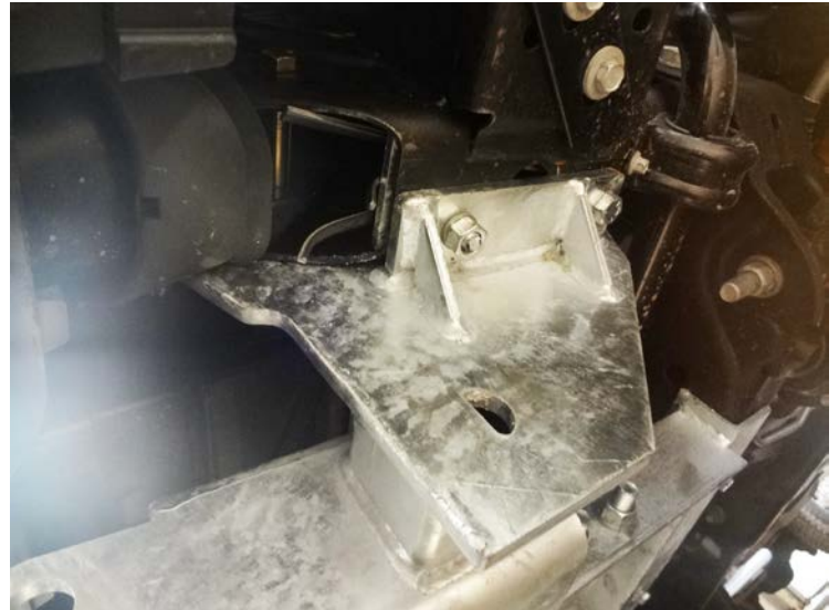
Mounting bracket (1) on Driver Side
