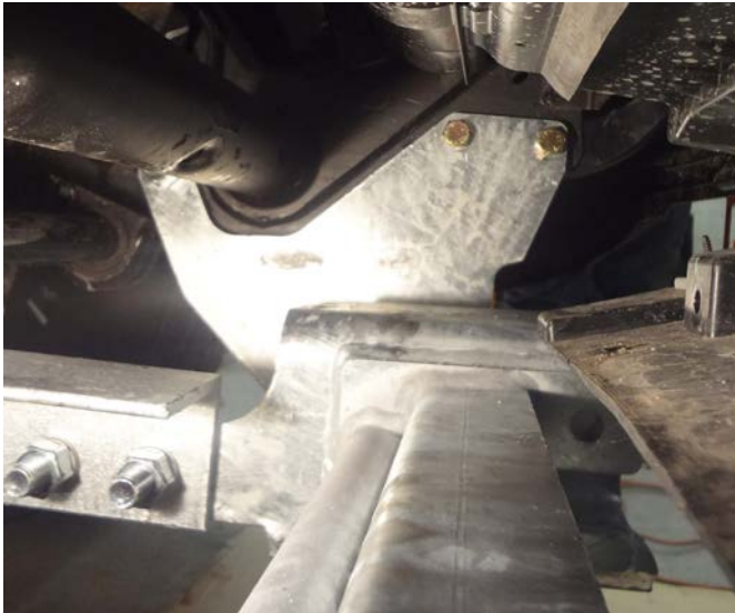
Mounting bracket (1) on Driver Side
