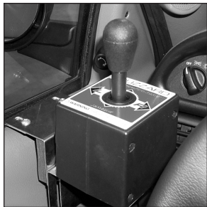
Straight Blade Joystick Window Mount Bracket P/N 61261
