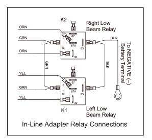
NOTE: If ring terminal wire does not reach battery, lengthen wire as required.
