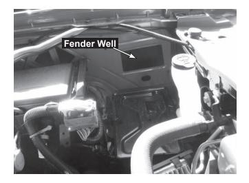
3. Install the edging material around the sides of the fender well as shown.
