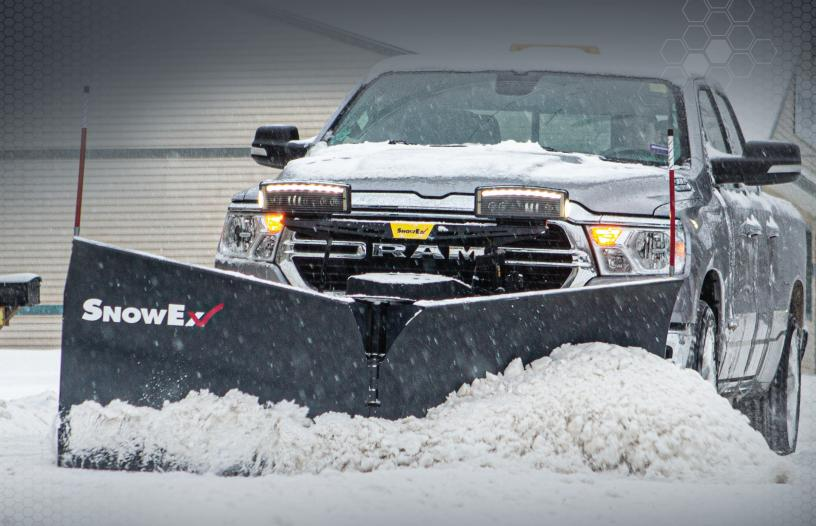
Redefine what your half-ton truck can do. The new SnowEx® RDV V-plows have the features and benefits of the larger plows but are specifically designed for half-ton trucks. They are constructed of high-strength, low-alloy steel, making them stronger and lighter than conventional steel. Available in powder-coated steel or stainless steel, the plows configure to varying vehicle heights for optimum performance on some of the most popular truck models.
