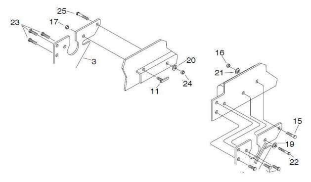
. Align the four holes in each side of the pushbeam with the holes in the mount plates. Choose the set of holes that will bring the pushbeam closest to the dimension shown below.
