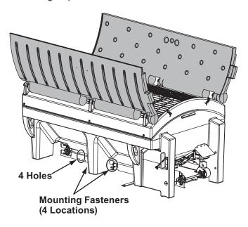
3. Position the vibrator so that the wire lead is up. Install the vibrator spacer plate into the four holes using 3/8" x 1-1/2" cap screws, washers, and 3/8" locknuts. Insert the 3/8" cap screws from the inside through the sill and into the vibrator. Secure with washers and 3/8" locknuts on the vibrator side as shown.
