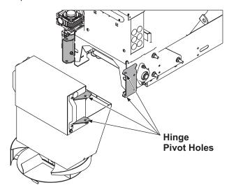
Insert a 1/2" x 8-1/4" chute pin on each side and secure with a 3/32" x 2-1/4" cotter pin.
