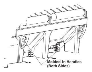
2. To lift the spreader into the truck bed from the ground, stand the spreader up on the feet at the rear of the spreader. The chute must be removed.
