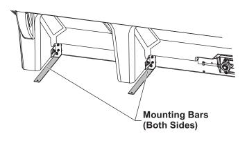
NOTE: Pay special attention when drilling or clamping dissimilar metals to aluminum bodies. Galvanic corrosion can occur if not handled properly. Contact vehicle manufacturer for recommended attachment practices.
