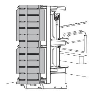
6. Do not leave an unsecured spreader standing on its feet. Lower the spreader so it is resting on its 6 legs and place spacers under the legs so the feet at the rear of the spreader are off the ground.
