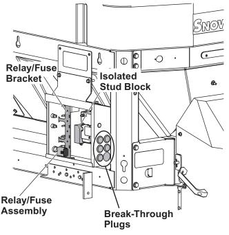
Electrical enclosure covers and relay/fuse assembly wires not shown.
