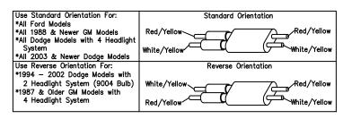
Figure 2. Vehicle Option Connector
