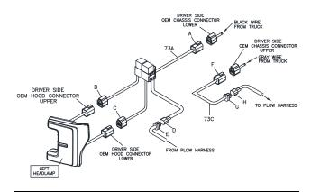
Figure 1. Ford Super-Duty LED Headlight Adapter Installation G13960
