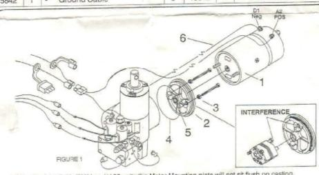
NOTE: On older E-60, E60H and V-66 units the Motor Mounting plate will not sit flush on casting, there is an interference problem. One of the bosses located on the new motor mounting plate interfers with a bolt head used to attach the Fenrier pump to the sump casting. Due to the height of the Fenner Pump one of the bolts will require that the head of the bolt be ground down to clear
