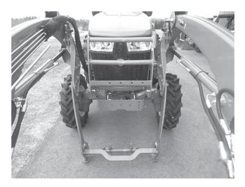
2. Remove the brush guard assembly (if equipped) by removing the fasteners from the brush guard arms. Save the fasteners for re-installation if the snowplow mount is removed.
