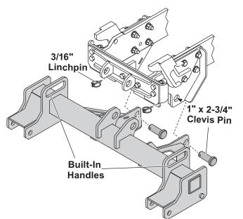
2. Install the removable push beam by inserting the 1" x 8" clevis pin through the lugs of the push beam and front mount assembly. Secure the clevis pin with the 3/16" linchpin.
