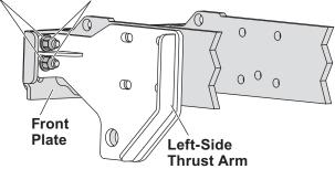
6. Place a 1/2" washer onto a 1/2" x 2" cap screw. Insert the cap screw and washer through the bottom rear hole of the left-side thrust arm. Secure with a 1/2" washer and 1/2" locknut. Tighten hand tight.
