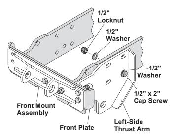
7. Repeat Steps 5–6 on the opposite side of the vehicle to install the right-side thrust arm.
