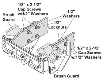
If the vehicle is not equipped with a brush guard, complete Step 8 using 1/2" x 2" cap screws in place of the 1/2" x 2-1/2" cap screws.
