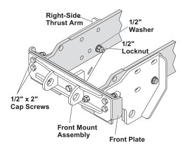
8. If the vehicle is equipped with a brush guard, re-install the brush guard over the right- and left-side thrust arms. Insert 1/2" x 2-1/2" cap screws with 1/2" washers through the brush guard, thrust arms, and vehicle frame. Secure the fasteners with 1/2" washers and 1/2" locknuts. Tighten hand tight.
