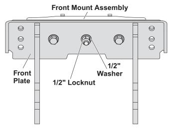
Place the left-side thrust arm against the frame. Insert two 1/2" x 2" cap screws through the front mount assembly, tractor front plate, and left-side thrust arm. Secure with 1/2" washers and 1/2" locknuts. Tighten hand tight.
