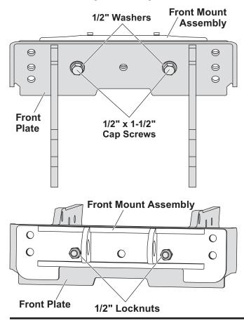
4. Insert a 1/2" x 1-1/2" cap screw through the center hole of the front mount assembly. Secure with a 1/2" washer and 1/2" locknut. Tighten hand tight.
