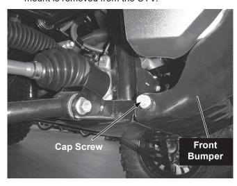
2. Position the skid plate assembly as shown below and secure it in place using an M10 x 45 cap screw and 3/8" washer on each side of the UTV. Do not fully tighten the cap screws at this time.
