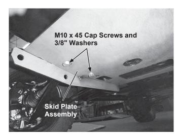
Tighten the cap screws (total of six) installed in Steps 2 and 3 to the recommended torque according to the torque chart.
