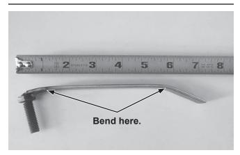
6. Place a 3/8" washer against the head of each 3/8" x 1-1/4" cap screw with handle. Insert a cap screw with handle inside the frame opening in each frame rail, and insert the fasteners down through the holes previously drilled in Step 5.
