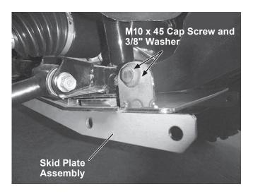
3. Align the four slots (two of which are shown in the photo below) in the bottom of the skid plate assembly with the weld nuts in the UTV frame. Insert an M10 x 45 cap screw and 3/8" washer into each skid plate slot and engage the weld nuts.
