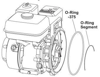
7. Reinstall the volute onto the rear bracket using the three volute screws. Reinstall the check valve onto the snout of the volute. The drive unit should be turned over a few times to check for clearance between the impeller and volute. A small amount of drag between the impeller and volute will cause no problem; however, if the drive unit will not turn over because of the lack of clearance, a shim may have to be used.
