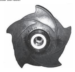
5. Install the impeller key shaft and impeller onto the engine drive shaft. Secure the impeller to the drive unit shaft with the impeller bolt gasket and the 5/16" x 1-1/8" hex flange cap screw. Tighten the cap screw until snug.
