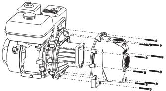
Reinstall the 10 body screws and secure with 10 lock washers and 10 nuts.
