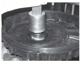
8. While the pump is completely disassembled, clean all of the reusable parts thoroughly, removing any traces of old gasket material and trapped or dried liquids that were run through the pump.
