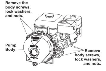
2. Remove the check valve from the volute. Remove the one upper and two lower volute screws, and remove the volute. Save all for later use.
