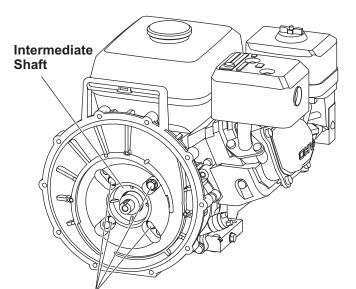
Rémove 4 bracket screws, rear bracket washers, and screw head O-rings.
