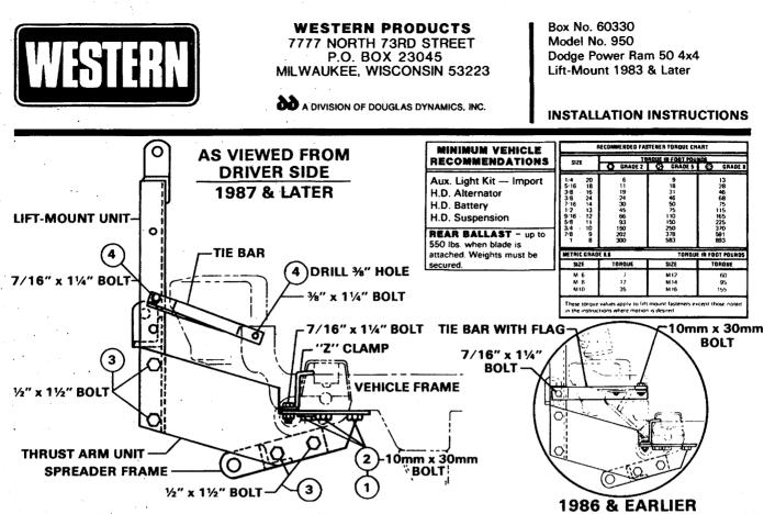
**IMPORTANT:** Read instructions before assembling. Bolts should be finger tight until the installation is completed to allow sufficient adjustment for aligning holes and locating parts to vehicle frame. Preventive maintenance can prevent accidents. Regularly inspect all components and repair or replace any worn, loose or damaged parts immediately. Remember to use standard methods and practices when attaching snowplow including wearing safety glasses during drilling.
