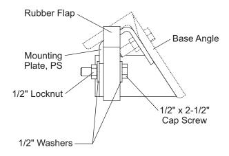
Insert the second 1/2" cap screw through the rubber flap and mounting plate weldment using the same washer and locknut assembly as mentioned above.
