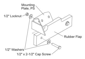
Place rubber flap against rear inside surface of the mounting brackets and align holes in flap and brackets.
