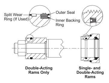
3. **For single-acting rams:** Slide gland nut over split bearing end of rod to prevent damaging seals.
