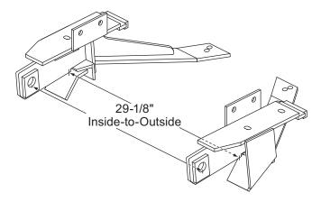
7. Check the inside-to-outside dimension between the connecting pin arms again. Repeat Step 6 as needed to obtain the 29-1/8" dimension while keeping the connecting pin arms parallel.
