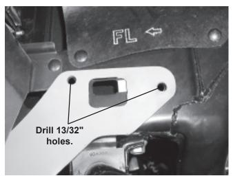
Insert two 3/8" x 1-1/4" cap screws with handles and 3/8" flat washers into the inside of the truck frame and out through the rear drilled holes. Attach a 3/8" locknut to each cap screw and hand tighten.
