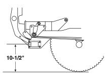
The recommended push beam height for this undercarriage assembly is 10-1/2" from the center of the push beam to level ground. DO NOT exceed 12-1/2" in height for this undercarriage.
