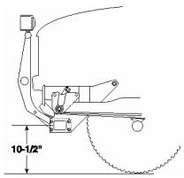
The recommended push beam height for this undercarriage assembly is 10-1/2" from the center of the push beam to level ground. DO NOT exceed 12-1/2" in height for this undercarriage.
