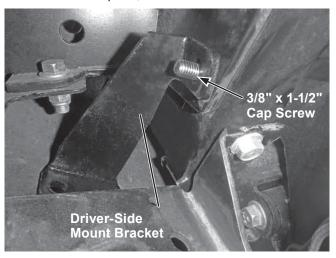
4. Install a 3/8" washer and 3/8" locknut to the cap screw and hand tighten.
