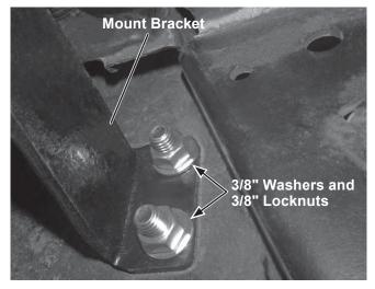
Clamp the rear of the skid plate assembly to the vehicle frame. Adjust as necessary so that the skid plate is centered. Tighten all fasteners installed above according to the torque chart.
