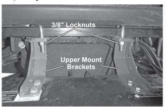
10. Use the rear mount holes as guides to drill 13/32" holes through the vehicle frame.
