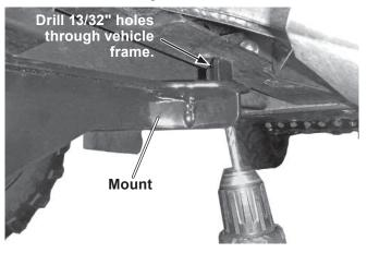
11. Place a 3/8" washer on a 3/8" x 2-1/2" cap screw and install it through the hole drilled in Step 10 and through the rear mount hole. Secure with a 3/8" locknut. Repeat for the opposite side.
