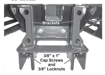
5. Using the holes in the tops of the brackets as guides, mark the locations of the four fastener holes on the brush guard.
