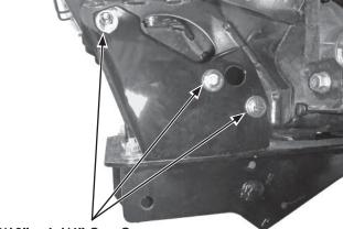
5/16" x 1-1/4" Cap Screws, 5/16" Washers, and 5/16" Locknuts NOTE: It may be necessary to adjust the front spring preload to increase the ride height. See the vehicle owner's manual for suspension adjustment procedure.
