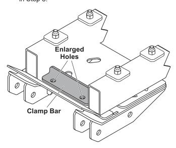
5. Place a 3/8" washer on each of two 3/8" x 1-1/4" cap screws. Install the fasteners up through the center holes of the skid plate assembly, vehicle frame, and clamp bar. Secure the fasteners with 3/8" locknuts. Hand tighten.
