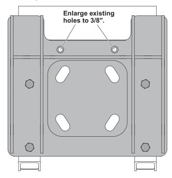
4. Install the clamp bar on the inside surface of the vehicles frame, positioned over the holes enlarged in Step 3.
