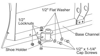
base channel, and one 1/2" x 1-1/4" cap screw, washer and locknut through the bottom hole in the holder and the base channel tab. Torque fasteners to 75 ft-lb.
