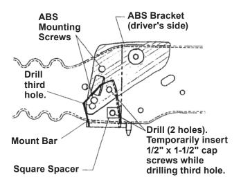
Use the formed plates as templates for drilling four 9/16" holes in each side of the vehicle frame. (Only three holes need to be drilled if the vehicle has a pre-existing slot.) Install two nut bars to the inside of each vehicle frame rail, aligning them with the drilled holes.
