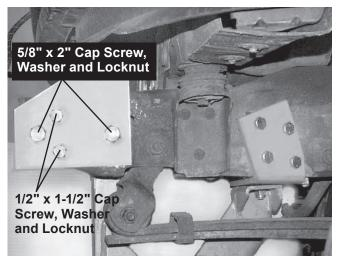
7. Loosely attach the mounts to the cross mount with one 1/2" x 1-1/2" cap screw, washer and locknut in the outer hole and one 5/8" x 2" cap screw, washer and locknut in the inner hole. Install flat washers against the slots in the mounts.
