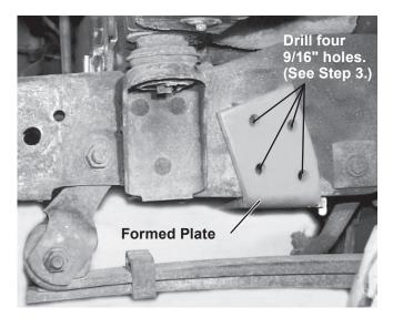
NOTE: Vehicles with an ABS bracket, as shown in diagram, require the following additional steps A through F to install the formed plate on driver's side.
