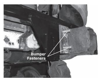
6. Align the large holes, and from the outside of the frame insert a 5/8" x 2" cap screw, two flat washers and a locknut on each side of the vehicle. Install a flat washer against the cross mount side plate and against vehicle frame. (Depending on the vehicle model and year, the hole locations for the 5/8" and 1/2" fasteners may vary from what is shown in the photos.) Install one fastener for each frame hole.
