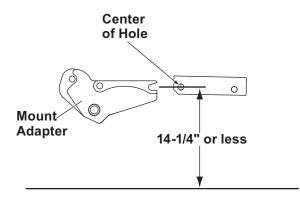
If measured height is 14-1/4" or less, no height adjustment is needed.
