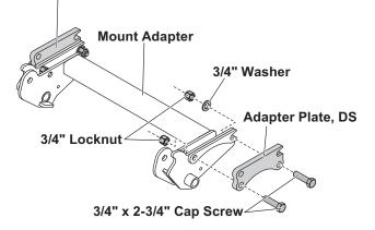
3. Repeat for the passenger's side. Tighten all fasteners according to the torque chart.
