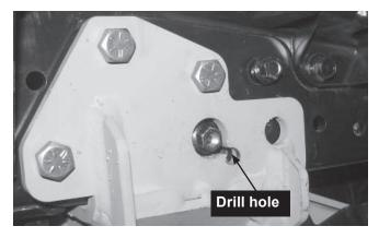
Reinstall the brake line bracket using a  $3/8" \times 1-1/2"$  cap screw and locknut in the drilled hole.
