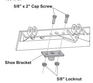
7. Determine the desired height of the cutting edge from the ground. Place the appropriate number of flat washers on the shoe and insert it up through the center hole in the shoe bracket and base angle. Secure with a linchpin.
