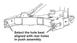
4. Lubricate and tighten all fasteners to 250 ft-lb.
