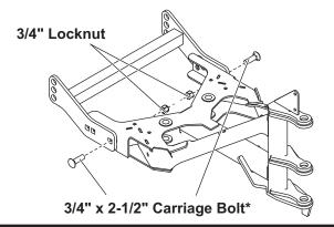
3. Align the rear holes in the pushbeam with the rear holes in the T-Frame and fasten in the middle position using two 3/4" x 2-1/2" carriage bolts\* and 3/4" locknuts. Tighten until assembly is secure, but do not torque at this time.
