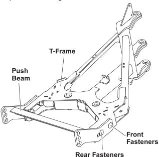
Select the hole in the rear of the T-frame that is aligned closest to the rear holes in the pushbeam.
