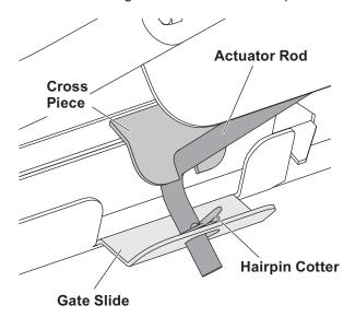
3. Insert the actuator rod through the main frame while sliding the upper push spreader handle assembly down onto the main frame. Fasten with 1/4" x 1-3/8" cap screws and 1/4" locknuts.
