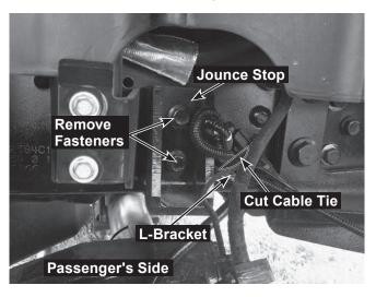
4. On the passenger's side, remove the jounce stop fasteners and the jounce stop.
