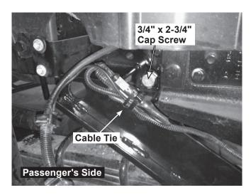
Cable tie the vehicle harnesses as shown. Apply the provided anti-chafing material to the harness or hoses if they come into contact with the thrust arm.
