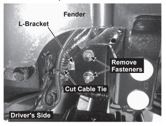
3. On the driver's side, remove the two fasteners shown above. Remove the plastic fender shown.
