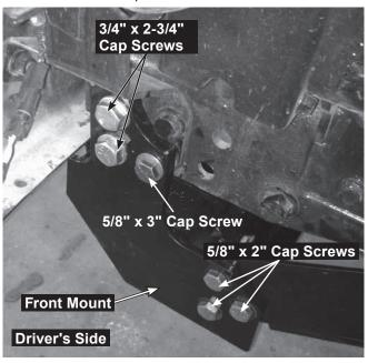
On both sides, loosely attach the corresponding thrust arm to the inside of the front mount using three 5/8" x 2" cap screws and locknuts. 8. Position the rear end of the passenger-side thrust arm as shown and attach using 1/2" x 2" cap screws and locknuts.
