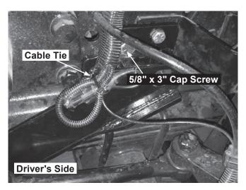
13. Secure the vehicle harnesses with cable ties as shown. Apply the provided anti-chafing material to the harness or hoses if they come into contact with the thrust arm.
