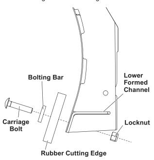
Adjust the position of the rubber cutting edge so that it extends approximately 1-3/8" beyond the bottom of the blade lower formed channel as shown. Tighten all the carriage bolts until the rubber starts to bulge.
