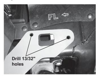
4. Insert two 3/8" x 1-1/4" cap screws with handles and 3/8" flat washers into the inside of the truck frame and out through the rear drilled holes. Attach a 3/8" locknut to each cap screw and hand tighten.
