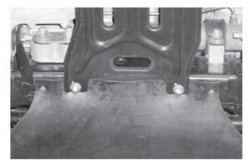
If the vehicle is not equipped with a transaxle skid plate, align the holes in the rear splash shield retainer and the tapered end of the splash shield with those in the vehicle frame cross member. Install two M6 x 25 mm cap screws (supplied with the mount) through the rear splash shield retainer and splash shield and into the cross member. Do not overtighten.
