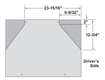
10. Position the splash shield on the vehicle so that the tapered end is toward the rear and the shield is on top of the mount and below the vehicle sway bar.
