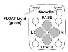
Pressing the four diamond-shaped buttons in the center of the control face will result in the blade movements described in the following table.
