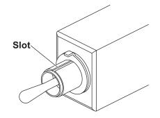
Install the switch from switch kit 40575 (Momentary ON-OFF-ON) into the plug with orange and black wires. The slot on the switch actuator shaft will line up with the orange replacement plug wire.
