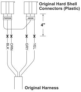
2. Remove 3/8" of insulation from the ends of the cut harness wires.
