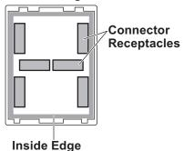
2. The plugs and switches are keyed to fit in the correct orientation. Ensure the body of the switch matches the plug before installing.
