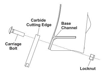
Align the two remaining cutting edges with the corresponding three holes outside of the center edge. Ensure that the carbide insert in each cutting edge is oriented in the "forward" direction.
