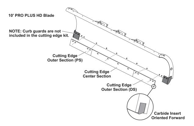
Insert the supplied carriage bolts through the cutting edge slots and through the base channel. Attach a locknut to each bolt and hand tighten.
