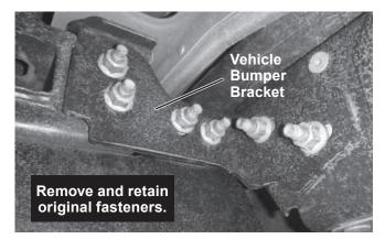
Position the pivot mount driver-side bracket assembly in place of the original bumper bracket. Use the fasteners retained in Step 1 to install the bracket assembly to the vehicle frame and bumper.
