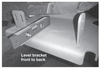
6. Level the passenger-side bracket assembly side to side. Check that the bracket is still level front to back. Hand tighten the fasteners.
