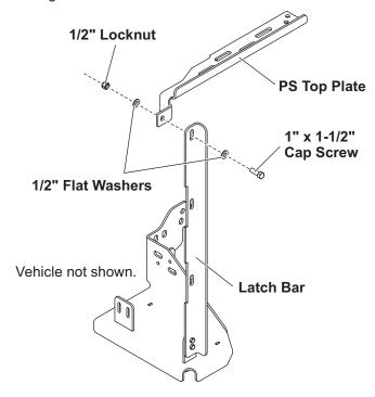
3. Use a level to confirm that the latch bar is vertical. If it is not, shift the top plate forward or backward along the bed rail until the latch bar is vertical. Clamp the top plate in position on the bed rail.
