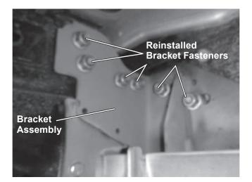
Install a 1/2" x 1-1/2" cap screw with 1/2" washer in each of the lower slots of the bracket assembly. Add a second washer and a 1/2" locknut on each cap screw, and hand tighten.
