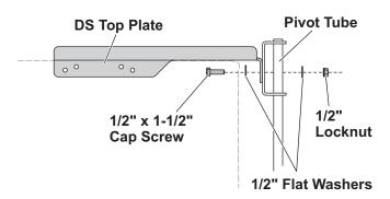
10. Use a level to confirm that the pivot tube is vertical. If it is not, shift the top plate forward or backward along the bed rail until the pivot tube is vertical. Clamp the top plate in position on the bed rail.
