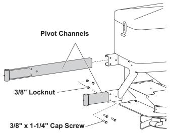
Slide the latch channels into the spreader frame on the passenger's side. Install each latch channel to the frame using three 3/8" x 1-1/4" cap screws, 3/8" flat washers, and 3/8" locknuts. Leave the fasteners loose for now.
