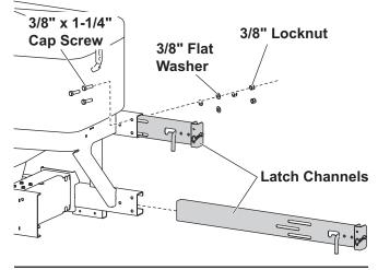
NOTE: The latch channels are slotted to allow for width adjustment of the pivot mount. To ensure a tight channel-to-frame connection, the supplied flat washers must be used with the fasteners installed in these mounting slots.
