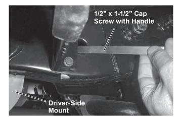
10. Place a 1/2" washer onto the cap screw, install a 1/2" locknut, and hand tighten.
