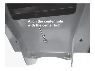
5. Clamp the skid plate assembly to the vehicle as shown. Place a 3/8" locknut on each of the four rear bracket cap screws. Hand tighten only.
