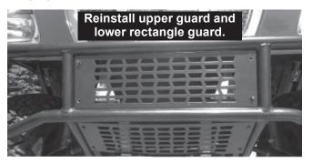
NOTE: After five to ten hours of snowplow usage, retorque all mount assembly fasteners.
