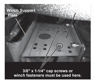
If a winch is not being installed, insert 3/8" x 1-1/4" cap screws through the indicated holes in the winch plate and through the holes in the forward frame cross member. Secure with 3/8" locknuts.
