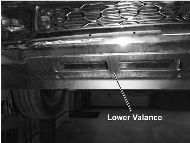
2. Starting on the driver's side, remove the compatibility bracket from the vehicle, if equipped. Retain the fasteners and bracket for reinstallation if the snowplow mount is removed.
