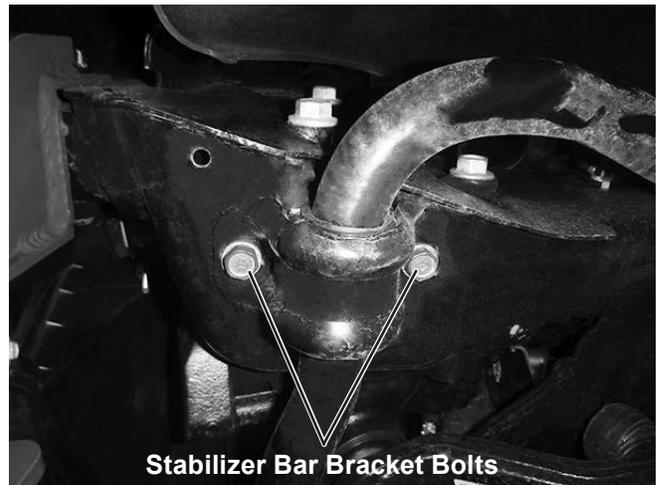
9. Install the mount brackets over the stabilizer bar. Insert two M10 x 1.50 x 40 cap screws through the stabilizer bar bracket and mount bracket. Apply a small amount of lubricant to the M10 cap screws, then push the stabilizer bar and brackets up against the frame. Thread the M10 cap screws into the corresponding holes in the vehicle frame. Use caution to avoid damaging the threads.
