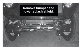
**For Gladiator models:** Remove the upper and lower splash shield brackets, if so equipped. Save the fasteners for reinstallation if mount is removed.
