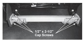
Check that the mount beam is level and make adjustments as necessary. Secure the mount beam by installing a 1/2" locknut on each 2-1/2" cap screw. Hand tighten the locknuts.
