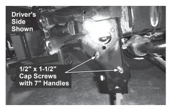
Place the driver-side mount plate against the underride structure, allowing the fasteners to protrude through the holes in the mount plate.
