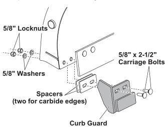
Repeat Steps 3 and 4 on the other end of the blade. 6. Fully tighten all cutting edge/curb guard fasteners to 150 ft-lb.
