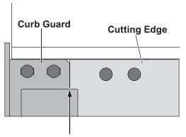
Make sure that the curb guard is flush against the cutting edge.
