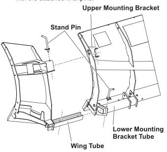
7. Tighten the mounting bracket fasteners to 75 ft-lb.
