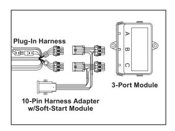
5. Mount the soft-start module in an area that receives good airflow, such as the cavity between the grille and the radiator.
