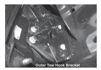
Remove the compatibility brackets from the frame, if so equipped (see illustration below).
