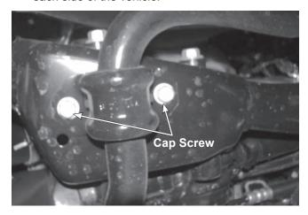
Position a stabilizer bracket between the bottom of the frame rail and the stabilizer bar retainer for both sides, facing inward as shown below.
