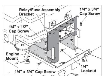
One of the two supplied fuse holders will serve as an isolated stud block. Install the isolated stud block to the relay/fuse assembly bracket using two #10 x 1/2" pan-head machine screws and #10 locknuts.
